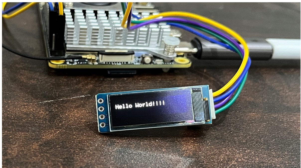
Fig. 5.22: Hello World!!!! on 128x32 OLED
