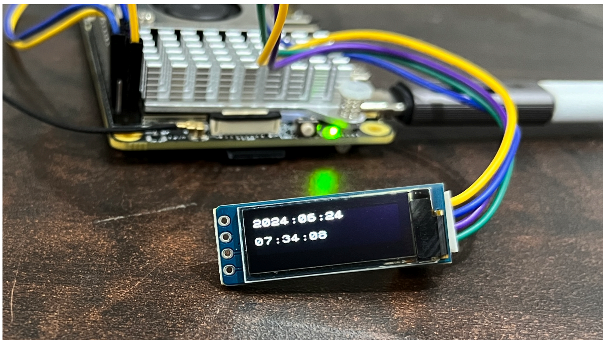
Fig. 5.24: Date &amp; Time on 128x32 OLED
