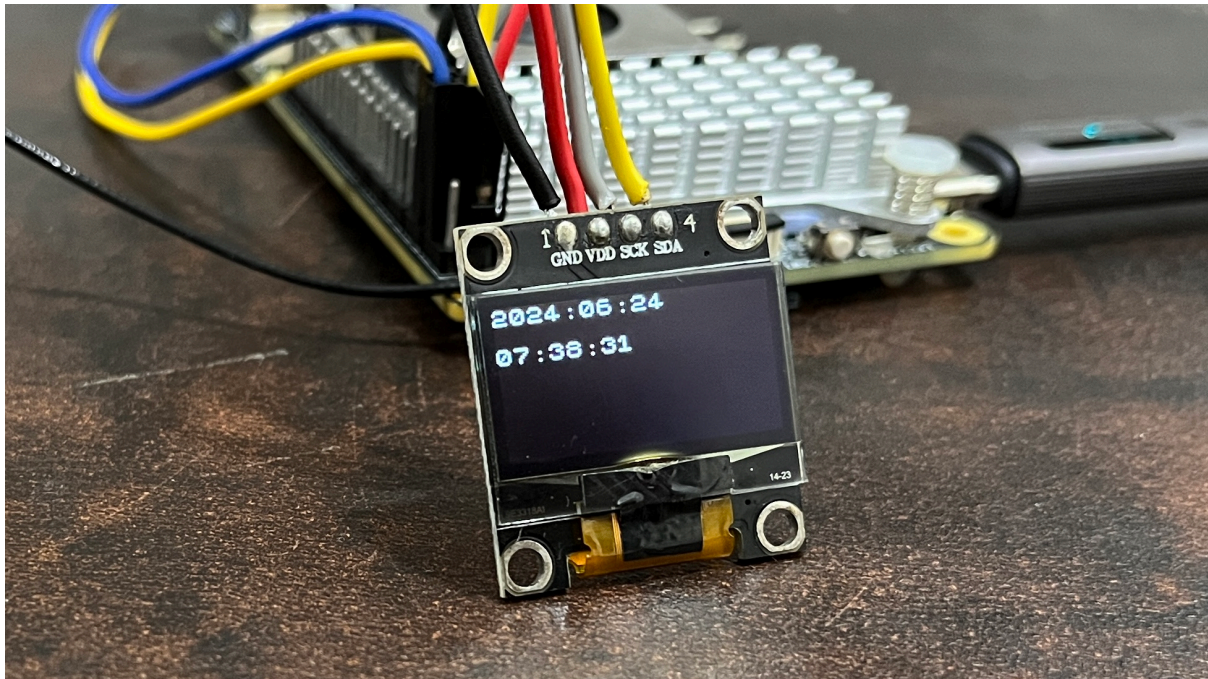
Fig. 5.23: Date &amp; Time on 128x64 OLED
