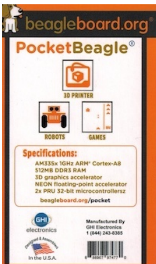
Fig. 3.3: PocketBeagle Package Insert back
